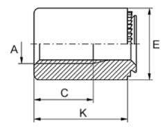
Female thread A = M5Height K = 10Min distance to edge = 4.0Outer diameter E = 9Plate thickness = 1.5 to 2.3Recommended bore diameter +0.05 = 6.00Thread length = 8.0
